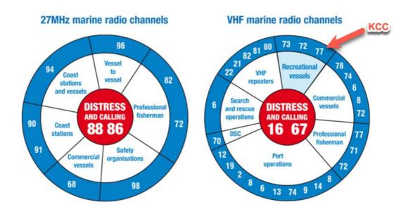
KCC prefers VHF radio Channel 77 when marine radio is used and monitored during KCC racing.
